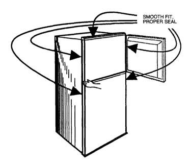
To adjust either door, loosen the hinge bracket screws, reposition the door then tighten the hinge bracket screws. To adjust up or down, add or remove washers from the lower hinge pin.
