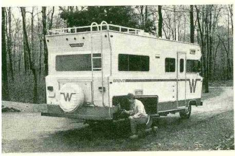
LARGE GLASS AREA gives rear lounge a three-way view. Our test vehicle had 4000-watt powerplant and 10,000 B.T.U. roof airconditioner (both optional). Cooler runs off powerplant on road, does excellent job without need for car air. Forced-air furnace keeps vehicle warm in coldest weather. Luggage rack and ladder proved to be useful options. Tire mount swings left to give access to compartment
