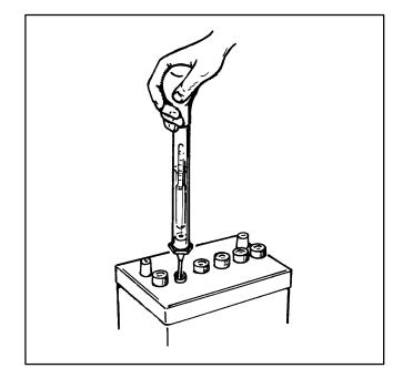
FIGURE 14. BATTERY CHECK WITH HYDROMETER
