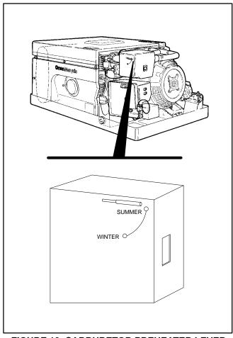
FIGURE 10. CARBURETOR PREHEATER LEVER (GASOLINE MODELS ONLY)
