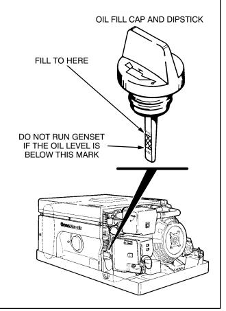
**FIGURE 12. OIL LEVEL CHECK**
