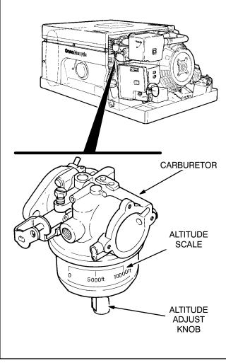
FIGURE 11. ALTITUDE ADJUST KNOB (GASOLINE MODELS ONLY)
