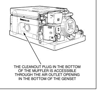
FIGURE 17. SPARK ARRESTOR CLEANOUT PLUG
