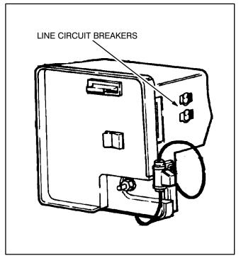
FIGURE 9. SET MOUNTED CIRCUIT BREAKER
