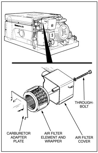
FIGURE 15. AIR FILTER ELEMENT AND WRAPPER
