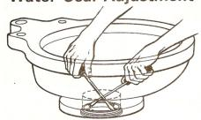
Each Traveler water closet has a visible adjustable ring (part 5) which screws into the plastic plate (part 6). When this ring is turned clockwise, the water seal is tightened. A counter-clockwise turn loosens the seal.
