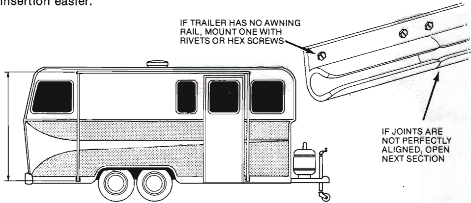
DISTANCE BETWEEN BOTTOM BRACKETS MUST BE THE SAME AS BETWEEN THE TOP BRACKETS, WITHIN 1/2"
