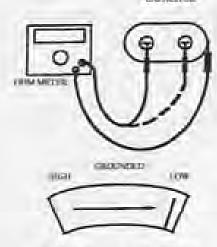
Indicator moves to the right side of the scale and stays there (indicating a completed circuit). The capacitor is grounded.
