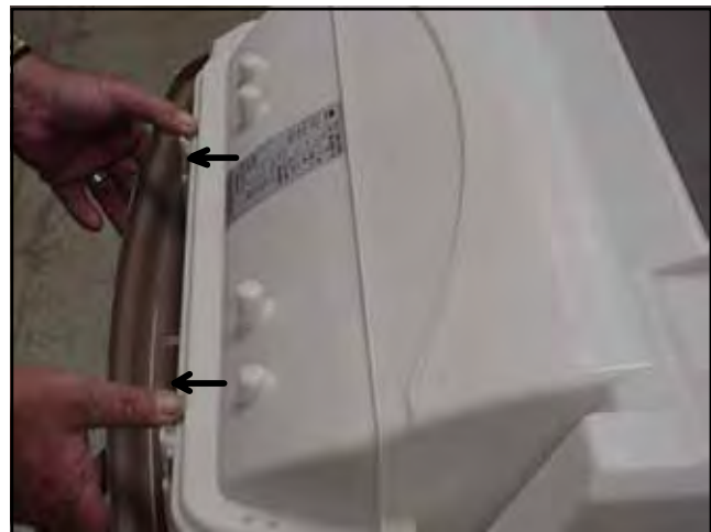
Figure 3-28 Upper Scroll Assembly Keeper Tab Release
