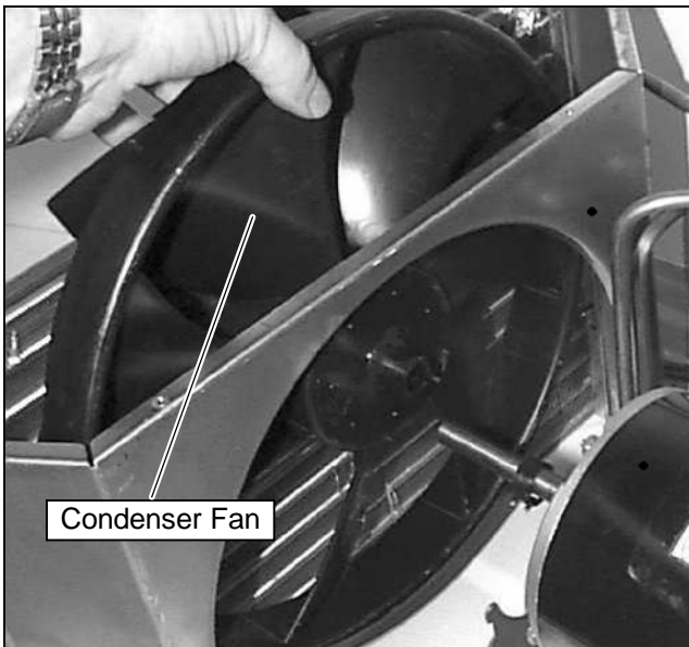
Figure 3-22 Condenser Fan Removal
